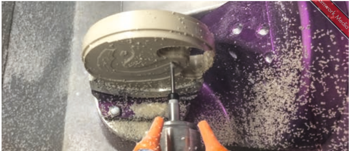
6 | Milling the secondary framework from unfilled PEEK (YuDent; Yunyi Medical).
